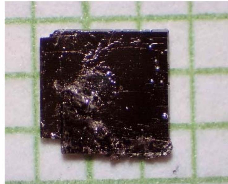
FIG. 1: Photograph of a single crystal of  $(\text{Ba}_{0.55}\text{K}_{0.45})\text{Fe}_2\text{As}_2$  on a mm grid. The crystallographic  $c$ -axis is perpendicular to the plane of the plate. Droplets of Sn flux can be seen on the surface.
