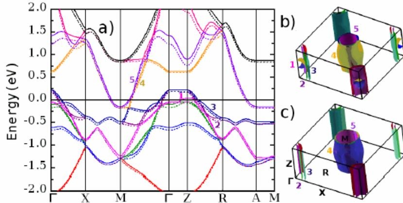
FIG. 2: (Color online) Calculated nonmagnetic electronic structures of LaO<sub>1-x</sub>F<sub>x</sub>FeAs. (a) energy band structures: the solid lines for the undoping while the dotted lines for the 5% F-doping (the Fermi energy sets to zero); (b) undoping: Fermi surface; (c) 5% F-doping: Fermi surface.
