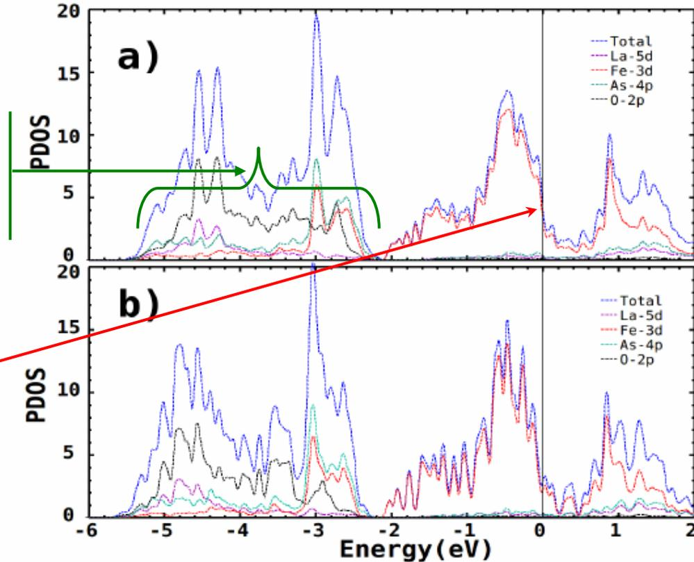
FIG. 1: (Color online) Calculated atomic orbital-resolved partial density of states of LaO<sub>1-x</sub>F<sub>x</sub>FeAs in nonmagnetic state. (a) parent compound LaOFeAs; (b) LaO<sub>0.95</sub>F<sub>0.05</sub>FeAs (5% F-doping). The Fermi energy sets to zero.
