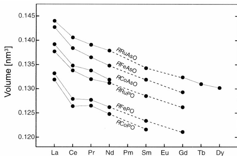
Fig. 1. Cell volumes of compounds  $RTPnO$  ( $T=Fe, Ru, Co$ ;  $Pn=P, As$ ) with ZrCuSiAs type structure.
