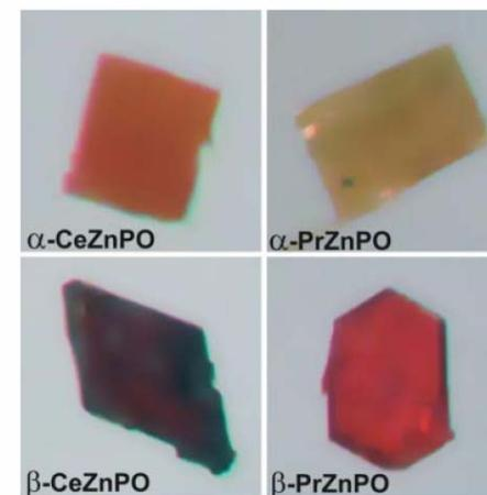
Fig. 1 Photographs of flux grown single crystals of the  $\alpha$ - and  $\beta$ -modifications of CeZnPO and PrZnPO. The edge lengths of the crystals are ca. 50  $\mu m$ .
