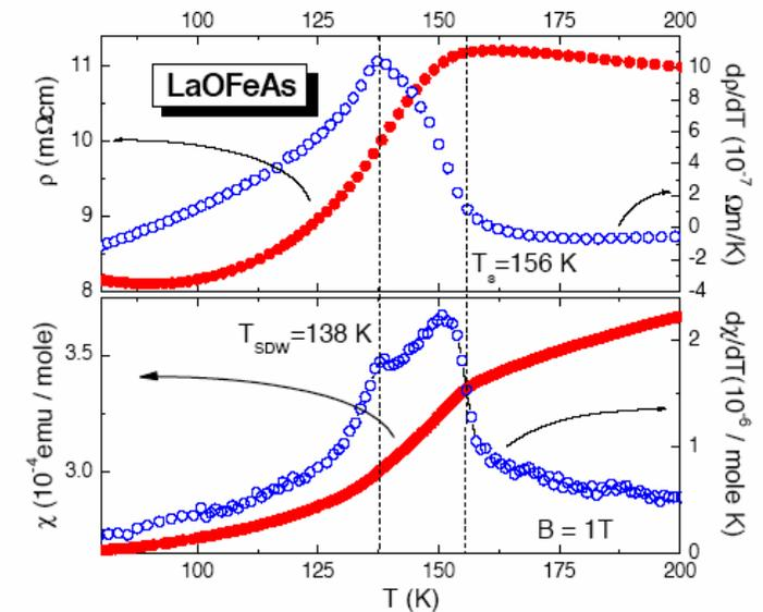
FIG. 4: Temperature dependence of (top) the electrical resistivity and (bottom) the magnetisation vs. temperature and the respective derivatives  $\partial\chi/\partial T$  and  $\partial\rho/\partial T$ .  $T_S$  and  $T_N$  mark the structural phase transition at 156 K and the SDW-formation at 138 K.
