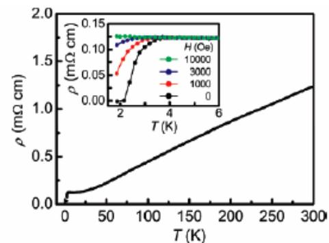
Figure 3. Temperature ( $T$ ) dependence of the electrical resistivity ( $\rho$ ) at 0 Oe. The inset shows the  $\rho$ - $T$  curves as a function of the magnetic field magnified in the temperature range of 1.9–10 K.
