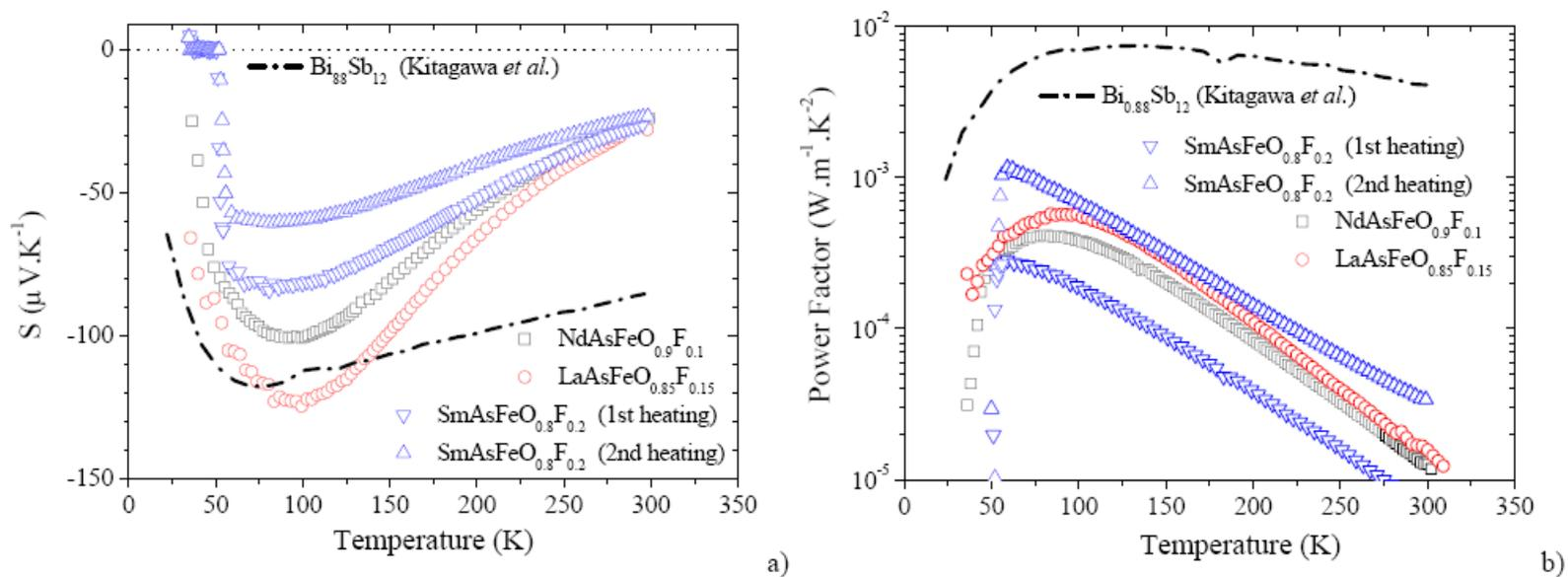
**Figure 2** Temperature dependence of a) the Seebeck coefficient and b) thermoelectric power factor of some  $\text{REFeAsO}_{1-x}\text{F}_x$  compounds. The dashed-dotted lines correspond to the data of  $\text{Bi}_{0.88}\text{Sb}_{12}$  reported in ref 9.
