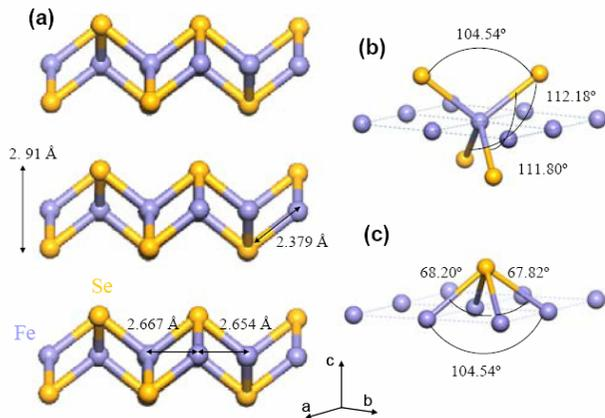
**Fig. 1** (a) Schematic diagram of the low-temperature orthorhombic crystal structure of  $\alpha\text{-FeSe}_{0.92}$ . Fe and Se ions are depicted as blue and yellow spheres, respectively. (b) and (c) Geometry of the  $\text{FeSe}_4$  tetrahedra and the  $\text{SeFe}_4$  pyramids with the three distinct Se-Fe-Se and Fe-Se-Fe bond angles indicated.
