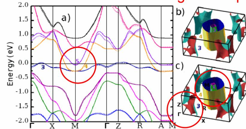
FIG. 3: (Color online) Calculated antiferromagnetic electronic structures of LaO<sub>1-x</sub>F<sub>x</sub>FeAs. (a) energy band structures: the solid lines for to the undoping while the dotted lines for 5% F-doping (the Fermi energy sets to zero); (b) undoping: Fermi surface; (c) 5% F-doping: Fermi surface. Note that here only the spin-up part is shown.
