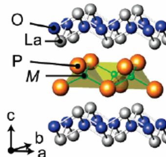
Figure 1. Crystal structure of  $\text{LaMOP}$  ( $M = \text{divalent transition-metal cation}$ ). The yellow polyhedron indicates the  $\text{MP}_4$  tetrahedron.  $\text{LaO}$  and  $\text{MP}$  layers are alternately stacked along the  $c$  axis.
