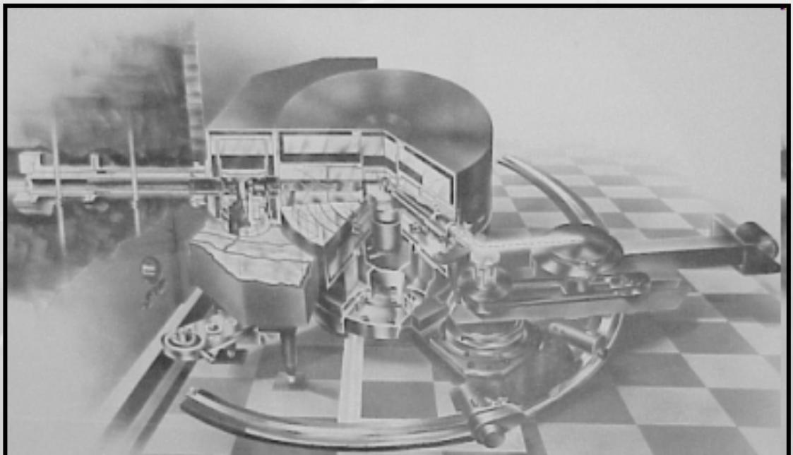
The Triple Axis Neutron Spectrometer
