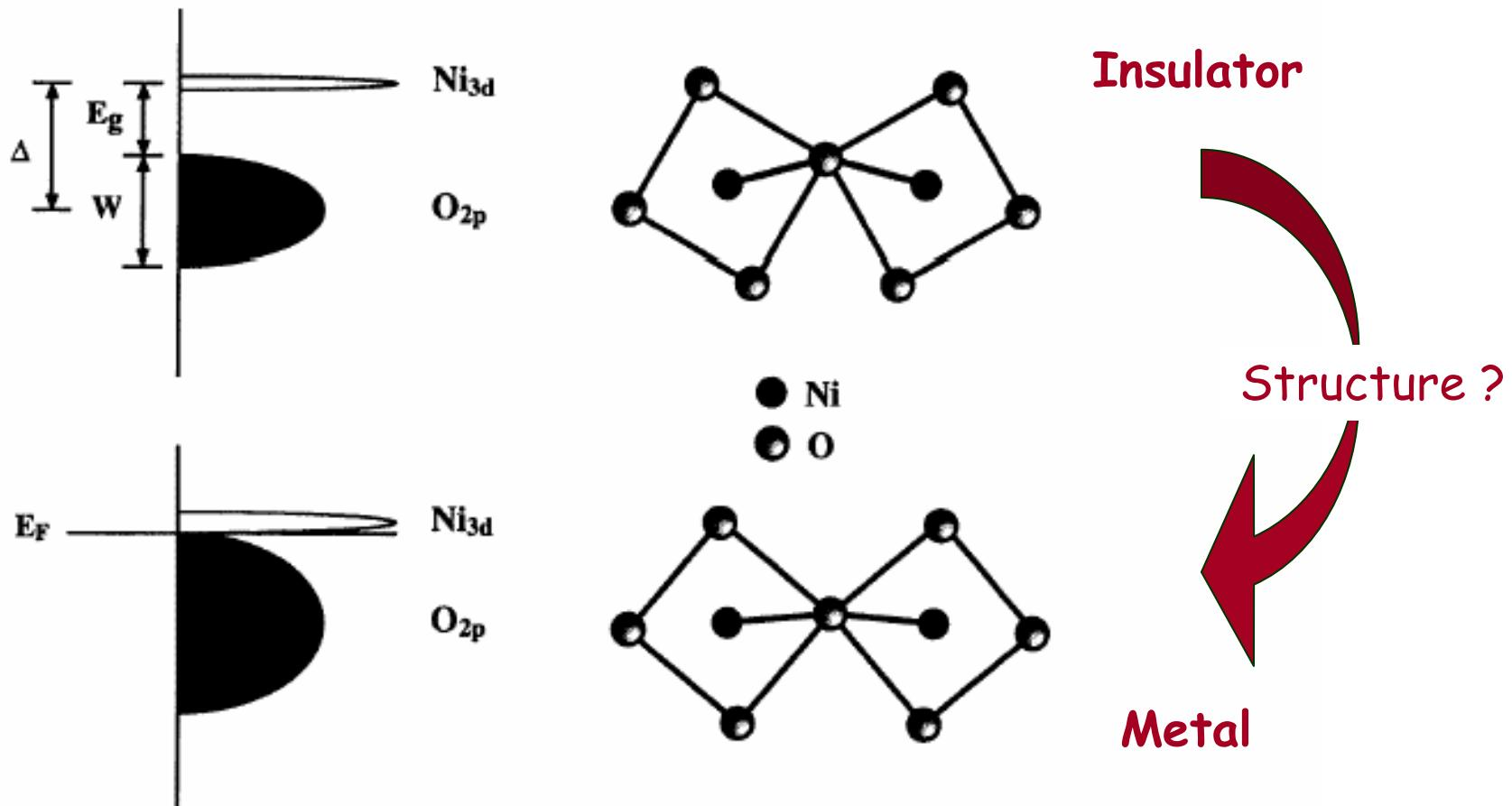
**Figure 15.** The M-I transition in the charge-transfer scheme. The narrowing of the O 2p-derived valence band below  $T_{M-I}$  would take place because of the less efficient overlap of the O 2p and Ni 3d orbitals produced by the decrease of the Ni-O-Ni superechange angle.
