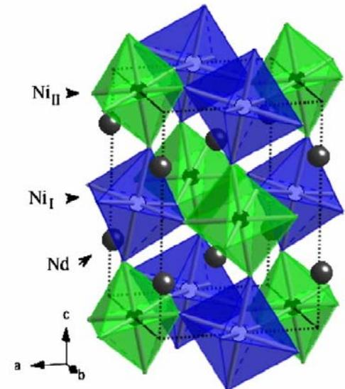
**Direct evidence**    Structural phase transition at  $T_{MI}$   $\rightarrow$  2 different types of octahedra
