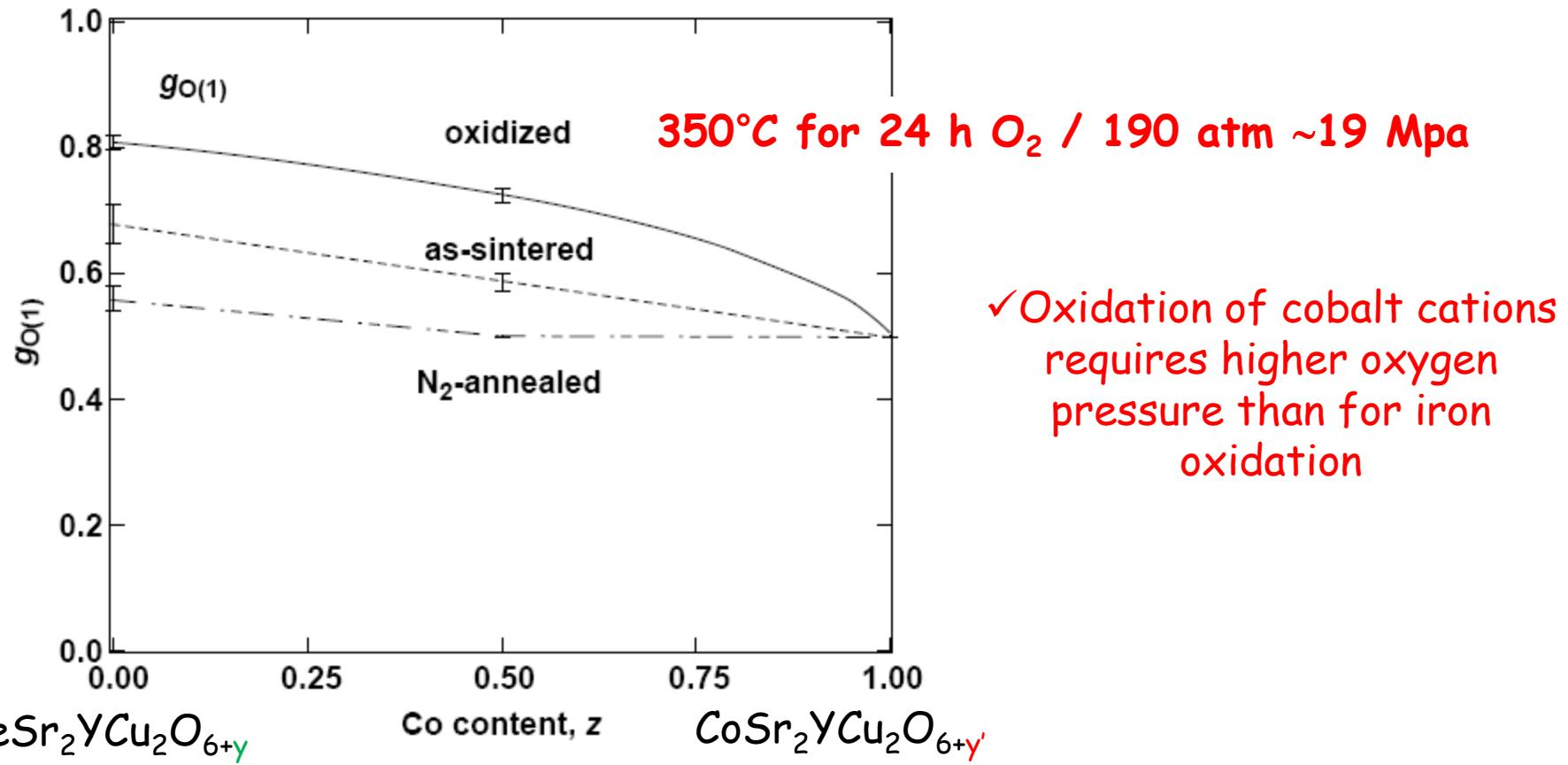
✓ Oxidation of cobalt cations requires higher oxygen pressure than for iron oxidation
