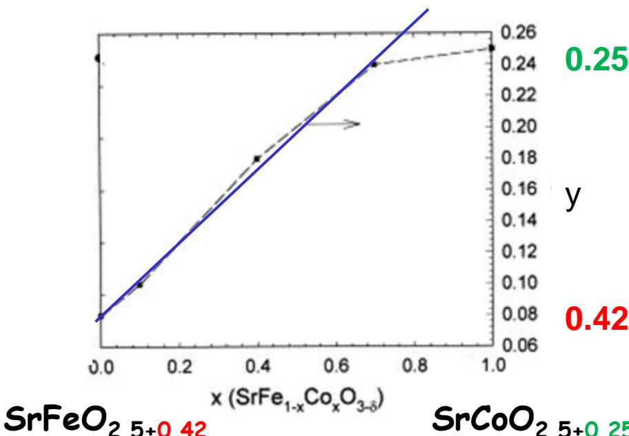
➤ The oxygen deficiency y increases continuously with the cobalt content until  $x=0.7$
