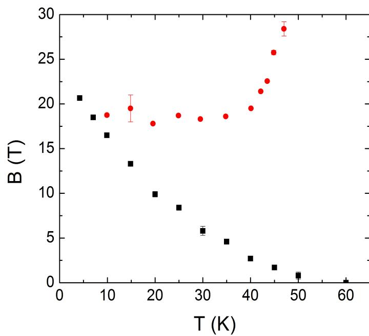
Phase diagram of the competition between SC and stripe order tuned by a magnetic field at  $T=0$
